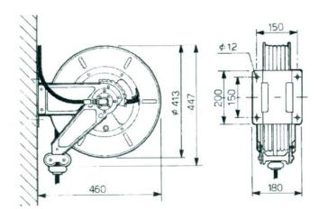
The automatic hose reels of the range V are suitable for transferring fluids at several pressures and temperatures.
